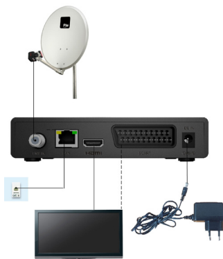
Example 3 – System with LAN connection
